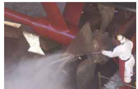
Removal of scale deposits and/or marine fouling
